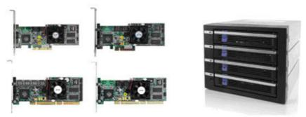
Our objective for this compatibility test is to confirm that our Areca 1110 / 1120 / 1210 / 1220 controller cards are fully compatible with ICY DOCK MB454SPF enclosure. We will be focusing on our controller and the enclosure's ability to handle Hot Plug, Hot Swap, and display LED activity properly as stated within ICY DOCK User manual.
