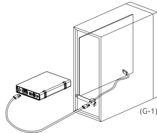
G. Optional 1 port eSATA PCI bracket w/ internal cables installation utilizing the MB559US-1S model device - (G-1)
