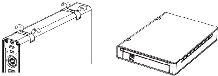
F. To position the device horizontally laying down, retract the foot stands by folding them inward and secured.
