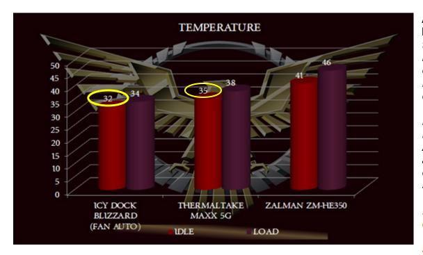
According to Hitechlegion - "We tested idle and load temperatures of our test drive in room temp of 20 degrees Celsius. Temperature readings were reported using AIDA64 at idle and max temps during a 50GB file transfer. The Icy Dock **Blizzard was** compared to the Thermaltake Max 5G which is
