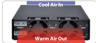
[ Dual Rear Fans & front airflow vents ]
